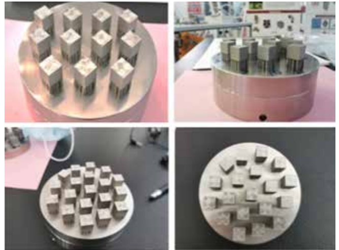
Fig. 11. Examples of samples printed using different L-PBF process parameters.
