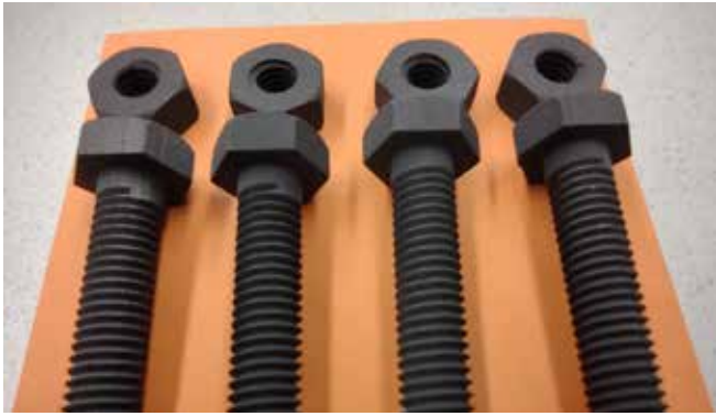
Fig. 10. Lithography-printed WC-Co M6 bolts and nuts.
