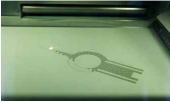
Fig. 3. L-PBF process: 3D printing of the metal parts for Hydro Impulse.
