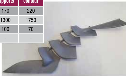
Fig. 4. Printing parameters and final 3D printed wing (compensated geometry).
