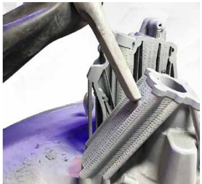
Fig. 5. Removing the support structure after 3D printing.
