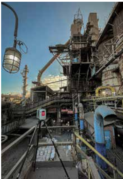
Fig.6. Scanning survey of a steel mill.
