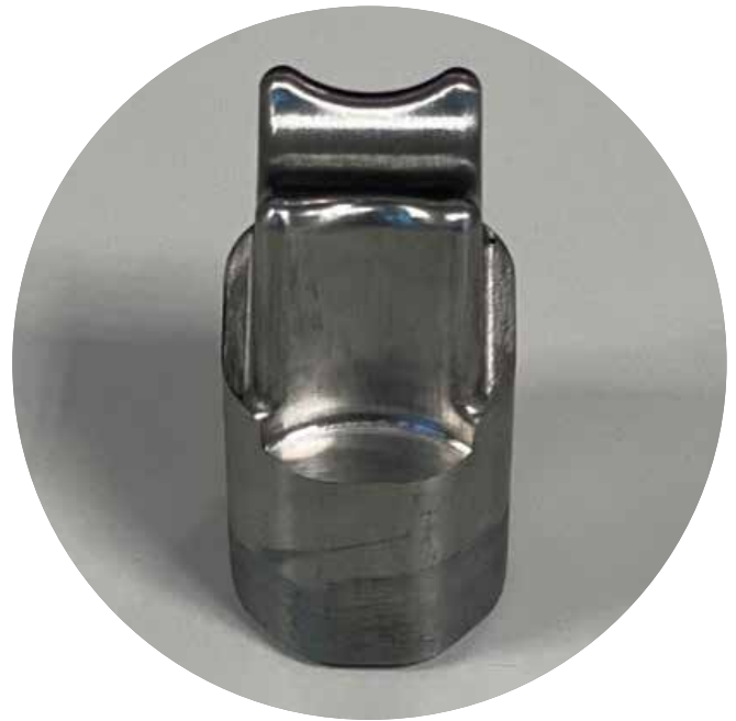
Fig. 13. Completed plug after machining.
