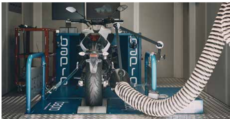
RICARDO – Dyno Roller Bench Test
