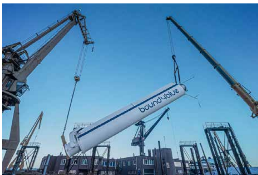
The largest suction sail in the world being installed at a shipyard. © bound4blue, 2021
