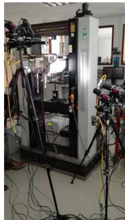
Fig. 4. Test configuration with a multi-camera system.
