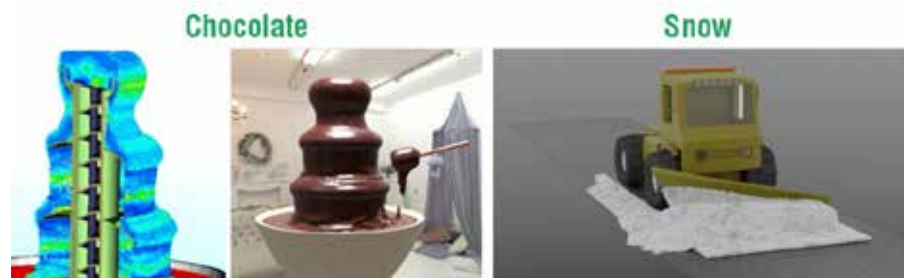
Fig. 2. The MPFI solver improves the simulation results for highly viscous fluids. Particleworks 8 also includes advanced snow models for more comprehensive analysis describing different snow textures and degrees of wetting.
