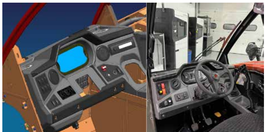
From the digital model to the printed ABS interior.
