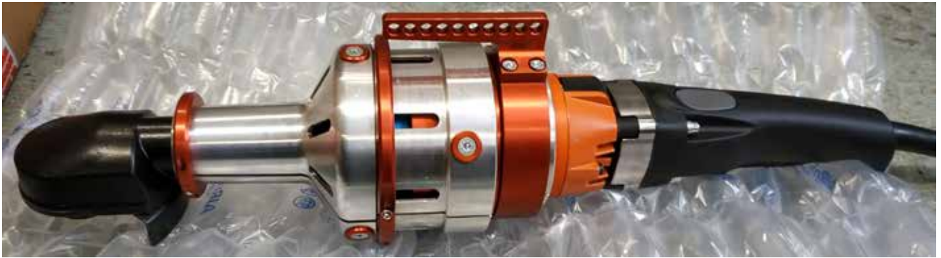
Fig. 2. First prototype of the grinder with the vibration reduction system installed.
