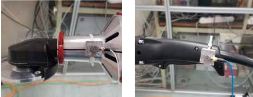
Fig. 7. Location of sensors placed on the handles of the modified grinder (front left and rear right).
