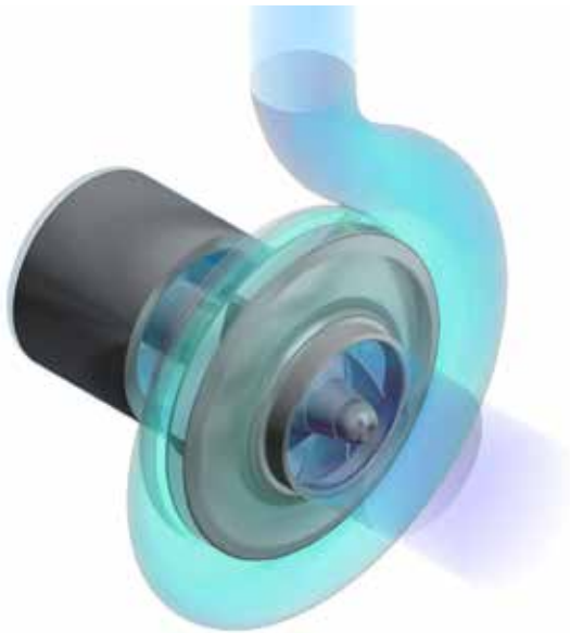
Fig. 3. A magnetic drive centrifugal pump.
