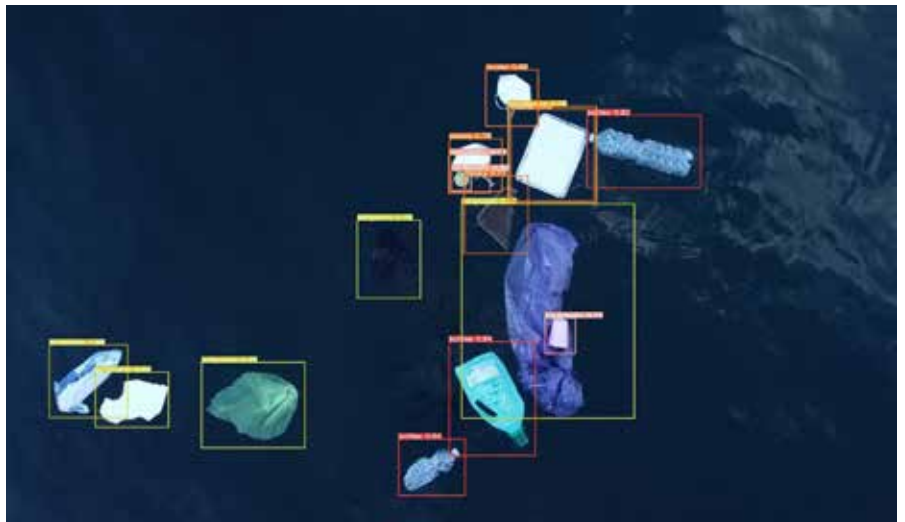
Fig. 1. Neural network trained in object detection can classify objects with an average accuracy of more than 90% Copyright: Green Tech Solutions.
