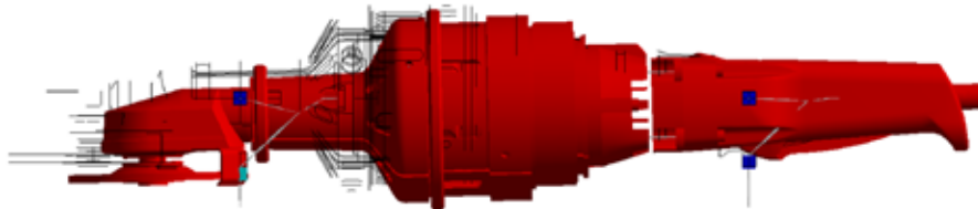
Fig. 6. Representation of the complete system's first vibration mode at a frequency of 1.51 Hz.
