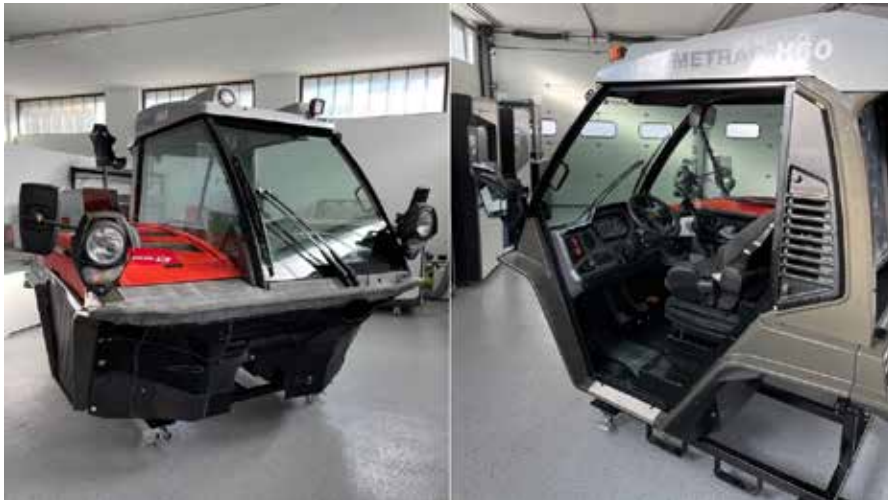
3D-printed vehicle cabin on show in Prirevo's showroom.
