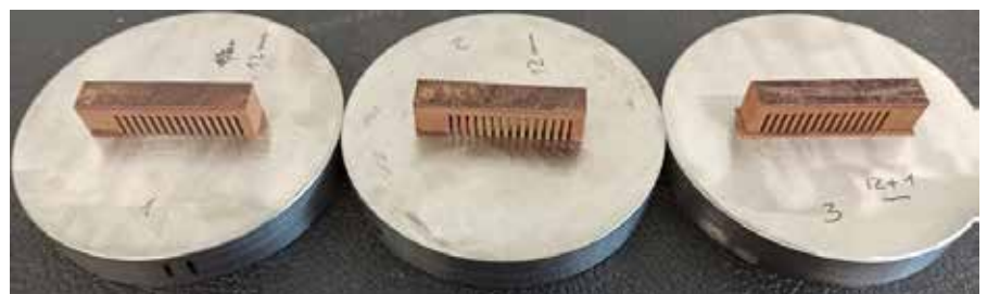
Fig. 5. SLM additive manufacturing specimens for calibration (courtesy of ECOR).
