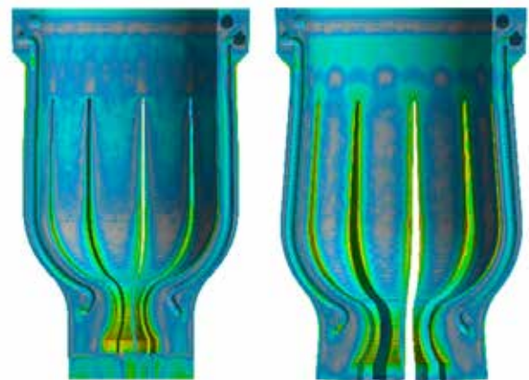
Fig. 9. Stress on the part in the as-built condition after process simulation. Right) job anchored to the platform. Left) after detachment of the part from the platform and the removal of supports.
